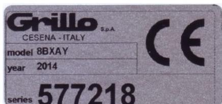
The rotavator is fitted with a nameplate on the frame with the serial number of the machine. Always state the serial number when ordering spare parts or asking for technical support.
